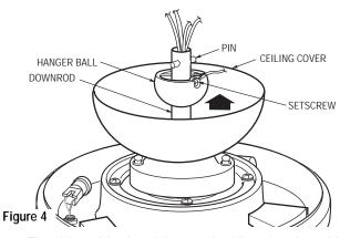
11. The blue, black, white, and yellow leads exiting the downrod are 80-inches long. Before installing the fan, measure up approximately 6 to 9-inches above the ball/downrod assembly. Cut off excess leads and strip back insulation 1/2-inch from end of leads.
